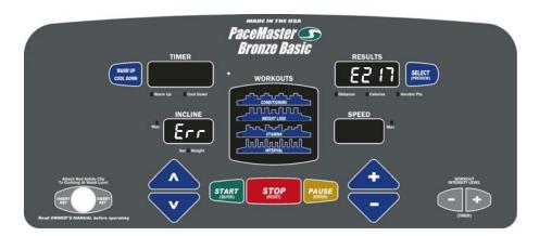
"Err" in the Incline Display - indicates a problem with the elevation system. Note: The treadmill will still function with the "Err" displayed in the incline Display, but the elevation system will not function. To determine the exact error code follow the procedure below.
